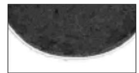
*Microscopic analysis of cross section of previously-tightened Tri-Star stud showing the thread root coating still intact.*
